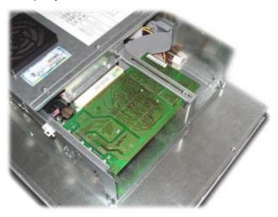
To ensure an optimal use of the board holder, we suggest that you put wide boards in the lower slots and narrow boards in the upper slots. Following picture shows this once more in detail.
