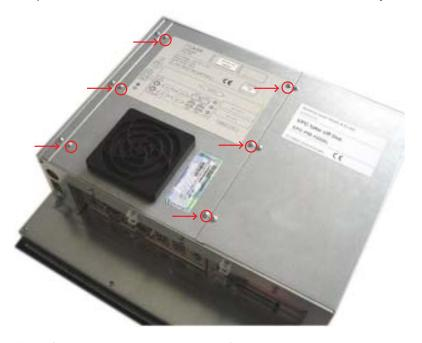
Then lift the enclosure and pull out the fan cable.
