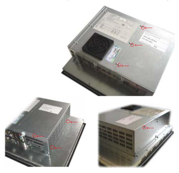
After removing 7 screws the enclosure can be lifted easily.
