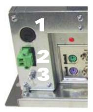
The power supply is carried out via a double-pole connector (Phoenix MST BT 2,5/2).
