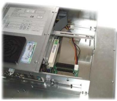
Remove the slot cover of the desired slot to insert your PCI-board.
