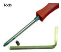
You can carry out the assembly with an Allan key 2,5 and a Phillips screw driver size 3.
