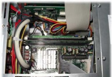
If a memory expansion is carried out the memory module is positioned vertically and pushed in, the fixing brackets snap shut.
