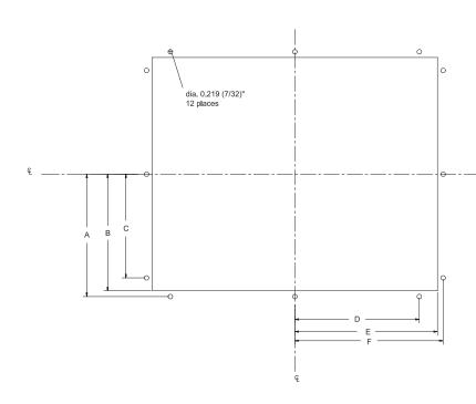
Template dimensions for FLI-150, FLI-150-TS, FPM-120, FPM-120-TS, FPM-150, FPM-150-TS, FPM-170 and FPM-170-TS models
