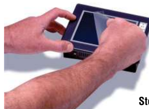
Step 3 Align the overlay with the screen and press the adhesive firmly into place
