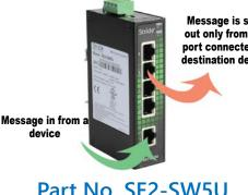
Message is sent out only from the port connected to destination device
