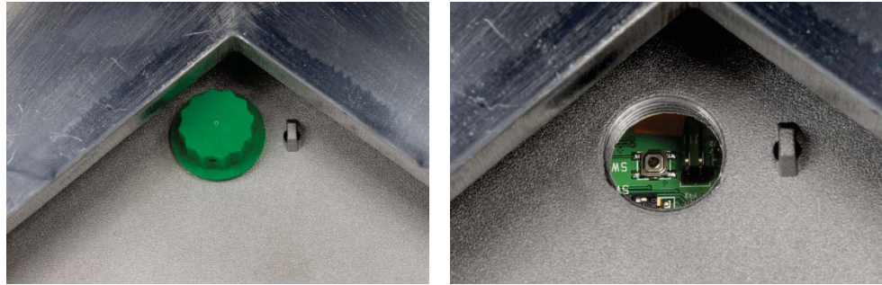
Figure 4-2: Access to Cal Button, BC30, BC3L, BC60, BC6L
