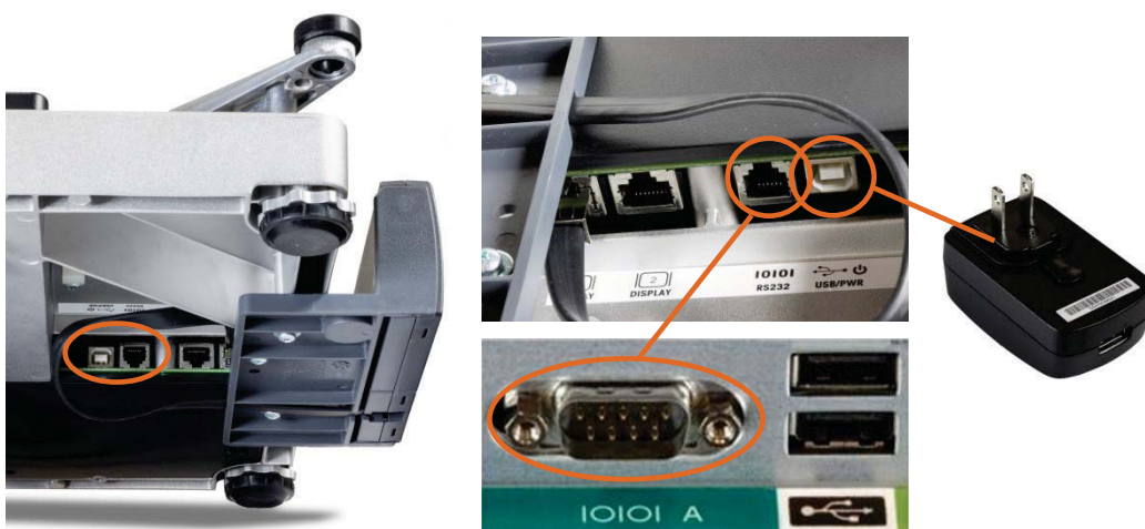
Figure 2-6: Serial Connections, Scale (left, top) and PC (bottom center); Power Supply (right)
