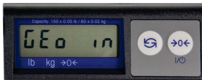
Figure 4-55: Basic (7-Segment) Display
