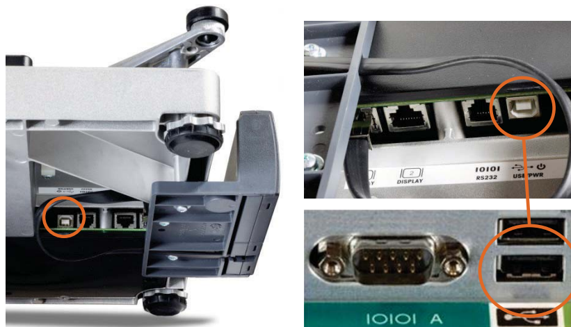
Figure 2-5: USB Connections, Scale and PC
