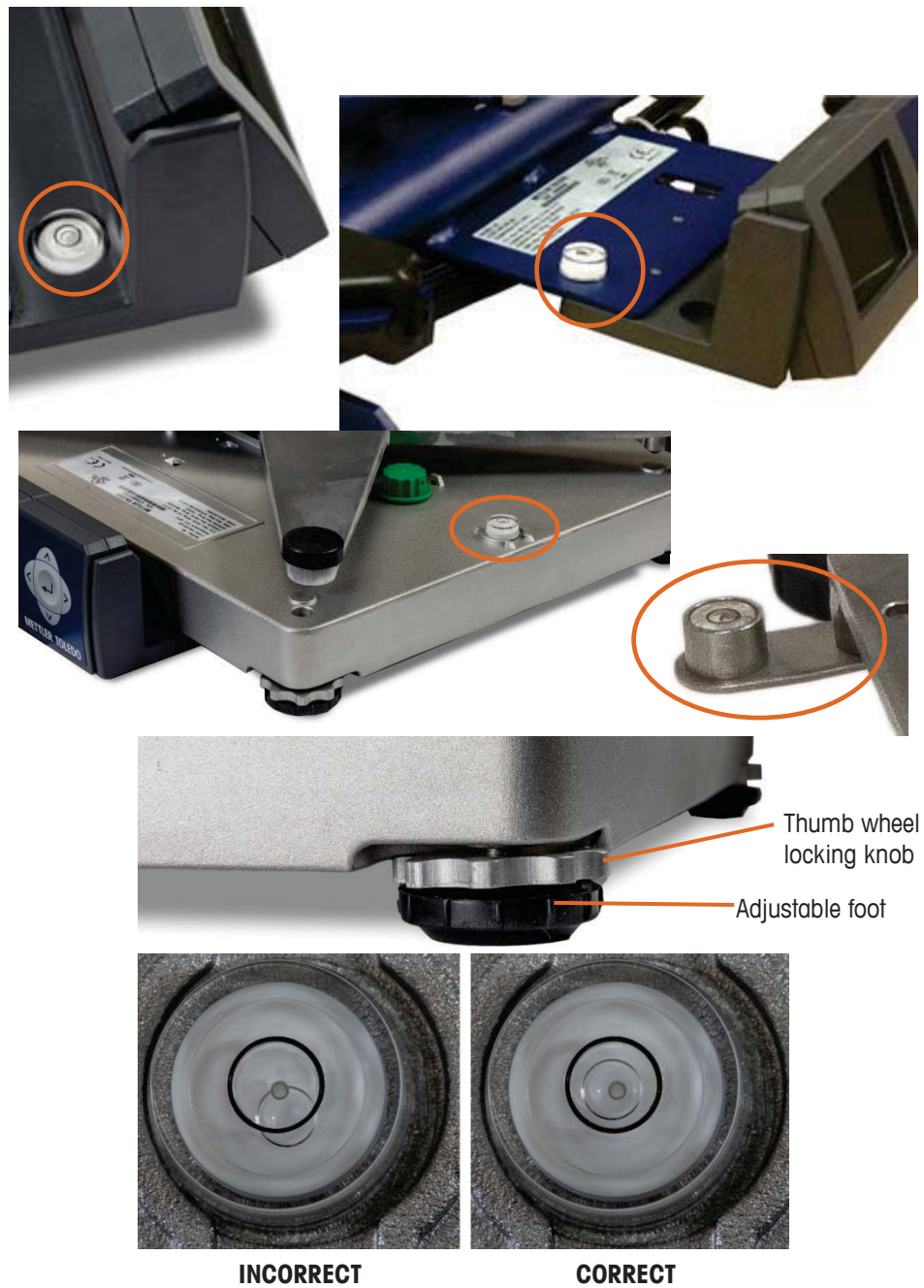
Figure 2-2: Leveling the Scale
