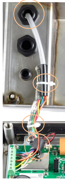
Figure 2-24: Analog Load Cell Pin Grounding and Ferrite Installation, IND236
