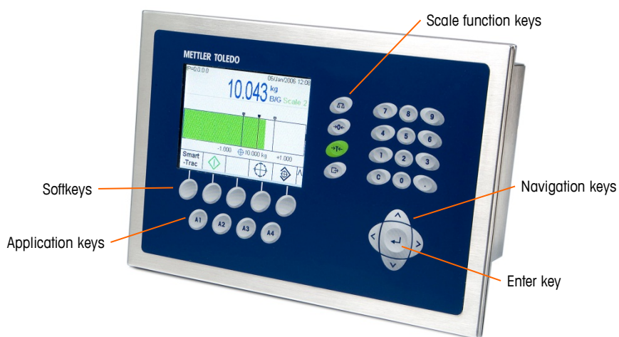
Figure 1-5: The IND780 Front Panel Layout
