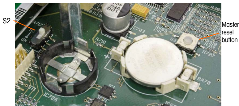
Figure 3-50: Main PCB, Master Reset Button and S2 Locations Indicated
