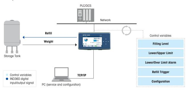
IND360 controls the refill valve while providing visualization on HMI. Cyclic and acyclic access to application status information and read/write of configuration using PLC interface, display or web interface. Redundant ring topology for PROFINET and EtherNet/IP is supported.
