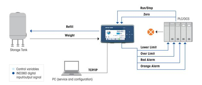
IND360 controls the refill valve and provides visualization on HMI. PLC access to status information and control functionality using digital I/O. Optional 4-20 mA weight output available for PLC/DCS connectivity. Configuration through web interface or display.
