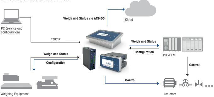
IND360 connects many different types of weighing equipment to automation controls such as PLCs or DCSs. It provides the ability to manage weighing applications that directly drive outputs for actuators and receive inputs from switches - see IND360 manuals for more details. IND360 is very easy to setup using the web interface that is accessed via a web browser such as Microsoft Edge or Google Chrome. When cloud connectivity is desired, choose the METTLER TOLEDO ACI400.
