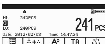
If the checkweighing result meets the specified checkweighing range requirement, the target value line  $\oplus$  will be highlighted, indicating that the current result meets the checkweighing range requirement.
