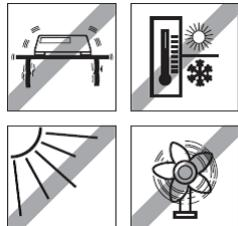
→ Select a stable, vibration-free and horizontal location for the scale.
