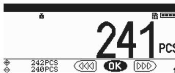
In big font mode, the soft keys line automatically disappears if no key is pressed for 2 seconds. The checkweighing status information is displayed instead.
