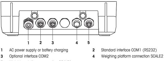
5 Weighing platform connection SCALE1
