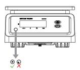
Only weighing platforms that have been levelled precisely horizontally provide accurate weighing results. Weights and Measures approved weighing platforms have a spirit level to simplify levelling.
