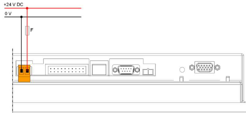
Fig.6-2: 24 V DC connection diagram
