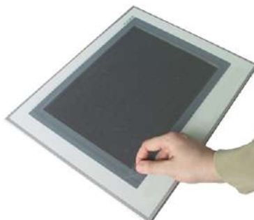
Fig.8-1: Detailed diagram 1: Remove the protective film
