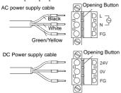
(4) After inserting all three pins, insert the Power Plug into the Power Connector at PL. Fix the plug with two minus screws.
