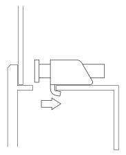
(4) Tighten the fastener screws equally in a diagonal pattern by using a Phillips screw driver. When tightening them, slowly increase the torque. (12 places)
