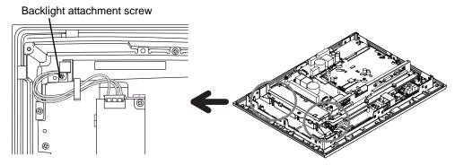
(7) Disconnect the cable of the backlight unit from the backlight connector on the inverter board, and remove it from the cable clamp.
