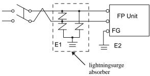
If the power supply voltage exceeds the FP unit's specified range, connect a constant voltage transformer.
