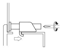
Do not use too much force, since it may damage the FP unit. A torque of only 0.8 N•m, are sufficient to tighten these screws.
