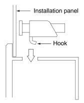
(3) Insert each of the fasteners as shown below. Be sure to pull the fastener back until it is flush with the rear of the attachment hole.
