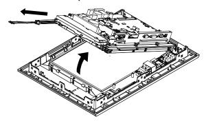
(9) Insert a new backlight unit into the port.
