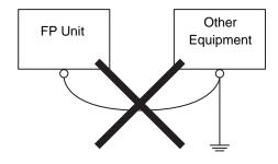
If this equipment does not function properly when grounded, disconnect the ground wire from the FG terminal.
