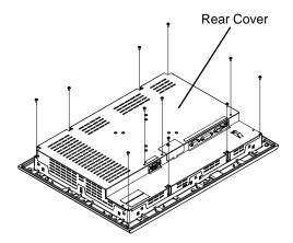
(4) Remove the rear cover of the module..
