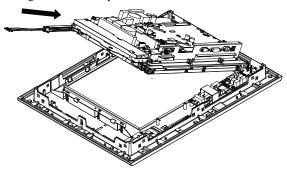
(10) Lower the LCD holder, connect the backlight cables to the backlight connectors, and secure the cables with the clamp. (Repeat the steps (7) through (10) for the other backlight unit.)
