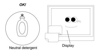
When the display surface or frame become dirty, use a soft cloth moistened with neutral detergent to wipe away any dust or stains.
