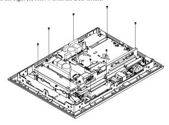
(6) Loosen the upper and lower backlight attachment screws.
