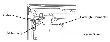
(8) Lift the LCD holder up as shown in the figure and pull the cable in the direction of the arrow. The back-light unit can be drawn out from the port.
