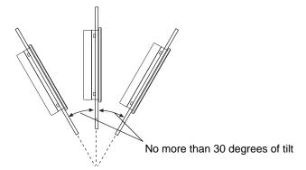
• When installing the FP in a slanted panel, and the panel face inclines more than 30°, the ambient temperature must not exceed 40 °C. You may need to use forced air cooling (fan, A/C) to ensure the ambient operating temperature is 40 °C or below.
