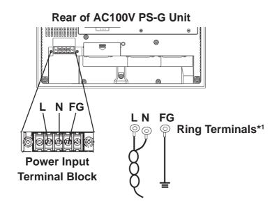
\*1 L : AC Input Terminal-live line N : AC Input Terminal-neutral line FG : Ground Terminal connected to the PS-G chassis Suggested Ring Terminal : V2-MS3 (made by JST)
