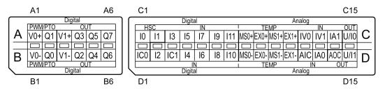
The table shows the group and signal names of the terminal blocks: **NOTE:** Confirm the connector label ABCD and the stamp ABCD on the unit before wiring.
