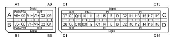
The table shows the group and signal names of the terminal blocks: **NOTE:** Confirm the connector label ABCD and the stamp ABCD on the unit before wiring.
