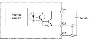
The circuit configuration of Q0 and Q1 is shown as follows: The circuit configuration from Q2 to Q7 is shown as follows: It is sink type
