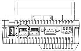
Do not confuse the RJ45 serial interface with the RJ45 Ethernet interface.
