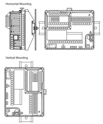
**NOTE:** Keep adequate spacing for proper ventilation to maintain an ambient temperature between  $0...50 \ ^{\circ}C (32...122 \ ^{\circ}F)$  for horizontal installation and  $0...40 \ ^{\circ}C (32...104 \ ^{\circ}F)$  for vertical installation.
