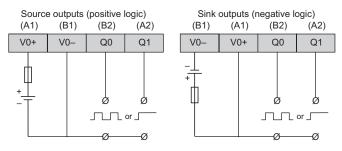
**NOTE:** Q0 and Q1 circuits are push-pull circuits. The following is the operation of the push-pull circuit at the Sink Output and the Source Output. Sink Output: +24(V) is output to terminal Q0, Q1 when the logic for Q0, Q1 is off Source Output: 0(V) is output to terminal Q0, Q1 when the logic for Q0, Q1 is off
