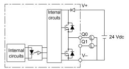
The circuit configuration of Q0 and Q1 is shown as follows: It is sink type
