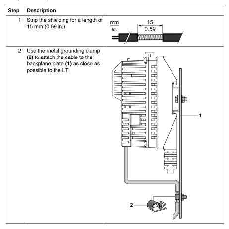
**NOTE:** The shielding must be clamped securely to the conductive backplane to ensure a good contact.
