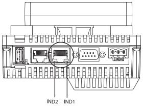
Do not confuse the RJ45 Ethernet interface with the RJ45 serial interface.
