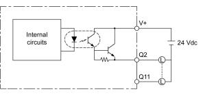
The circuit configuration from Q2 to Q11 is shown as follows: It is sink type
