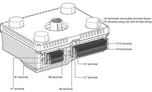
The figure shows the pin assignment of the terminal blocks:
