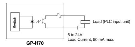
If the current level becomes higher than the rated value, the internal fuse will blow (melt). When connecting a load, be careful that the current flow is not excessive.
