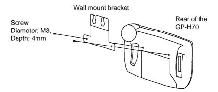
2. Screw the GP-H70 bracket's placement screws (shown) into the wall.
