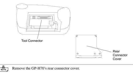
Be sure to turn the GP OFF before inserting or removing a connector from the Tool Connector socket. (i.e. the power cord has been unplugged).
