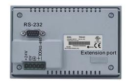
5-PIN terminals: Wire gauge: 12-24 AWG / Torque: 4.5 lb.-inch
