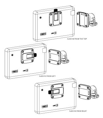
The quick release tab should point in the opposite direction from the direction you will slide the display out of the mount.
