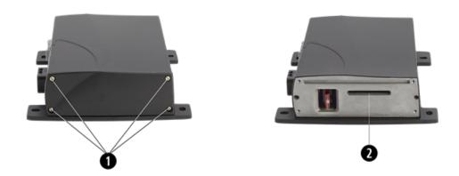
2. Insert the AG-815 blade connector (2) into the radio expansion slot of the TM-200 Module. Use the long screws provided with the A**G**-815 to fasten the it to the TM-200 Module.
