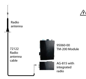
**CAUTION** – Wireless, cellular, radio and GNSS signals can interfere with each other. For best performance, mount antennas at least 1 meter away from each other.
