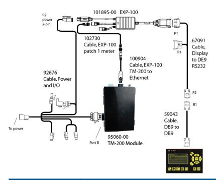
This diagram shows the connections for the Hardi 5500 controller with serial variable rate and radar output.
