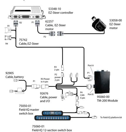
**Part Number Description** 53058-00 **EZ-Steer motor** 53348-10 EZ-Steer controller 62257 **EZ-Steer motor** 75050-01 Field-IQ master switch box 75060-01 12-section switch box (optional) 75742 EZ-Steer cable 92676 TM-200 Module power and I/O cable connected to port B
