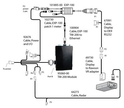
This diagram shows the connections for the Rawson™ drive module with serial variable rate and radar output.
