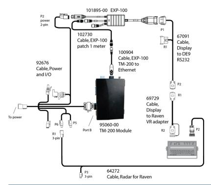
This diagram shows the connections for Raven with serial variable rate and radar output.
