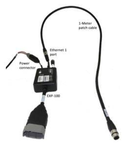
3. Connect the TM-200 Adaptor cable (100904) to the other end of the 1-Meter Patch cable
