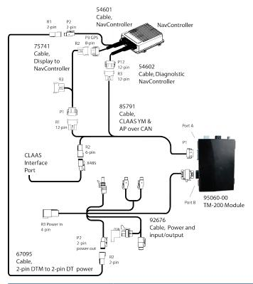
Use this diagram to connect the CLAAS Jaguar forage harvester.
