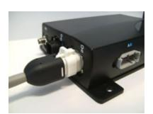
Ensure the cable is fastened into the cable clip next to the port on the rear of the display.
