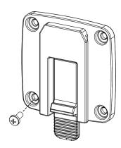
**Note** – Do not attach the display plate with the quick release tab pointing down. This will cover the connection port or USB port.
