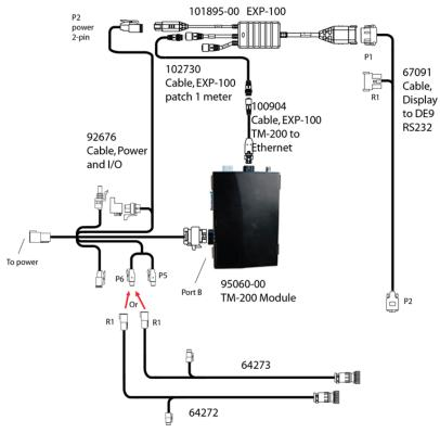
This diagram shows the connections for third-party controllers with serial variable rate and radar output.
