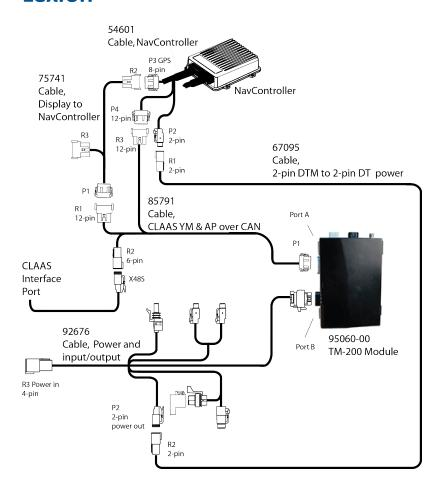
Use this diagram to connect the CLAAS Lexion grain harvester.
