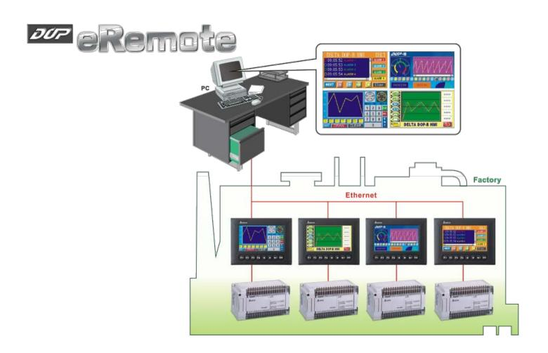
eRemote is used to view and check the HMI screen at the production site and to control the manufacturing process via the Ethernet.
