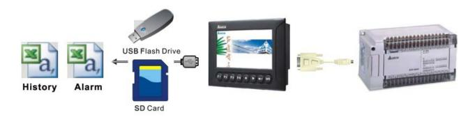
Much project screen data can be saved on the USB flash drive simultaneously and transferred to the HMI.
