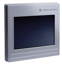
The ETT 352 is a touch operating panel with a 3.5" TFT color display. The resistive touch screen serves as the input medium for process data and parameters. To save energy, the display is deactivated in sleep mode. When the screen surface is touched, the terminal is activated and then deactivated a few minutes after the last input.
