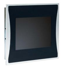
The ETT 312 is a touch operating panel with a 3.5" TFT color display. The resistive touch screen serves as the input medium for process data and parameters. To save energy, the display is deactivated in sleep mode. When the screen surface is touched, the terminal is activated and then deactivated a few minutes after the last input.
