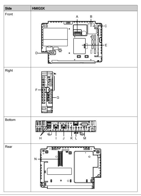
A: Auxiliary output/ Speaker output interface (AUX)
