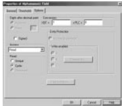
Reminder of the requirements specification: The amount of dough must be between 2800 and 3000. If the amount is not within these limits, the display will switch to red.
