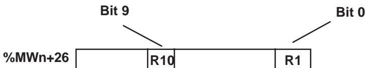
If for the same key, the lighting and flashing bit are at 1, the indicator is flashing.
