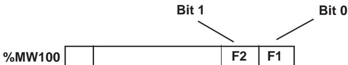
Bits B0 and B1 are associated with the F1 and F2 command keys.
