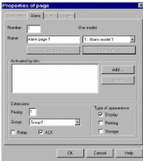
Select Type of action: **Display** (type of action when the alarm is triggered).
