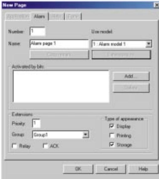
The XBT-L1000 software allows you to define the properties of the alarm pages (Figure 1-15).
