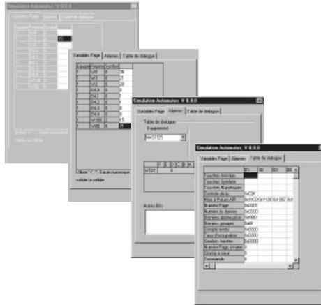
XBTL1003/L1004 software offers the option of simulating all the operator dialogue applications from the design office without the use of graphic terminals and PLCs.
