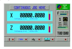
All of them use OEM screens that have been created on a PC using the Fagor Wgdraw application software and have been sent out to the CNC using the Fagor WinDNC application software.
