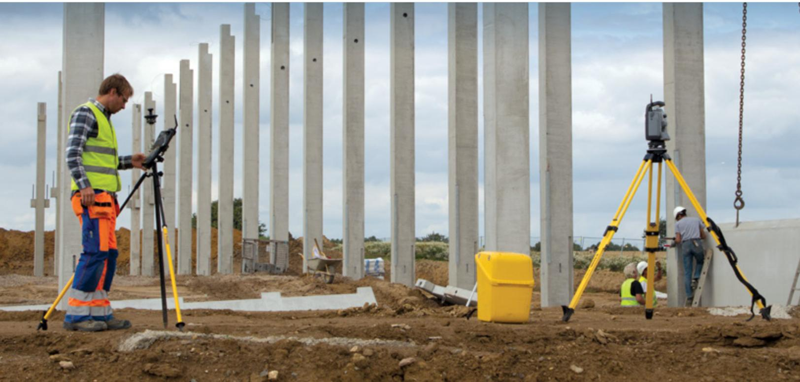
Trimble VISION technology integrates calibrated digital cameras with Trimble S9 and S7 total stations, as well as the Trimble SX10 scanning total station. These instruments have the ability to collect survey data, stream video from the perspective of the instrument, and capture panoramic still images. Trimble Access field software overlays survey data on the streaming video, which enhances your field productivity when operating the instrument robotically.
