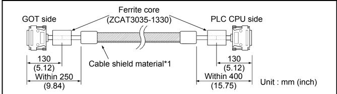
\*1 The back aluminum foil side of the cable shield material (shield side) should be exposed. (Refer to section 6.3.2 (1) (b))
