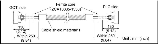
\*1 The back aluminum foil side of the cable shield material (shield side) should be exposed.
