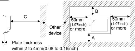
Part A size: 130mm (5.12inch) or more is necessary for the GOT coupling cable bending radius.
