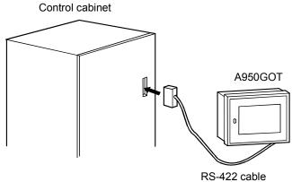
RS-422 cable to connect the GOT and the computer link unit must be prepared by the user.
