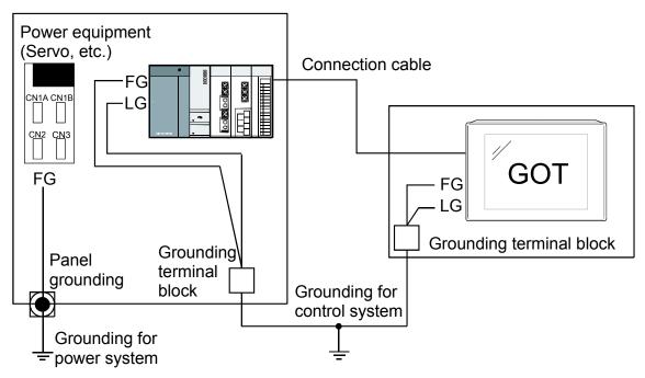
\* For control system grounding, apply single-point grounding for one system.
