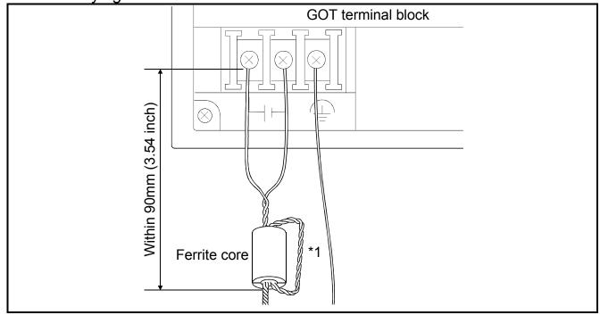
\*1 Wrap the power wire around the ferrite core.
