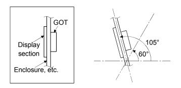
The GOT will be deteriorated earlier if it is used at the mounting angle other than the above. Therefore, the temperature inside the enclosure should be within  $40^{\circ}$ C.
