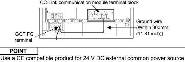
for GOT. The EMC test run by our company was confirmed with the same panel components as the DENSEI-LAMBDA type JWS 50-24 or DLP120-24-1
