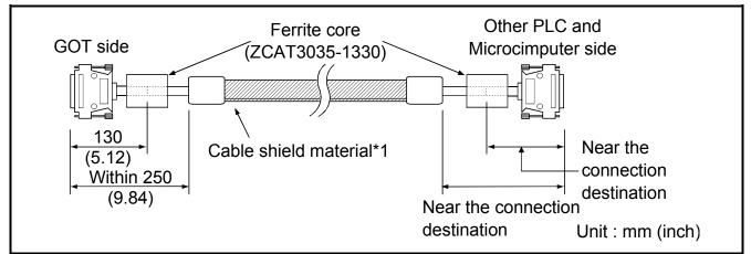
\*1 The back aluminum foil side of the cable shield material (shield side) should be exposed. (Refer to section 6.3.2 (1) (b))
