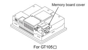
3 Set to OFF the protection switch in the memory board.
