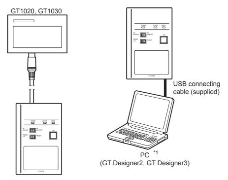
\*1: When GT10-LDR is connected to a PC via the USB hub, the power supply of the USB hub must be supplied by the AC adopter of the USB hub.
