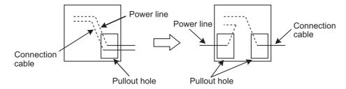
Keep the power line and communication cable inside the duct at least 100 mm away from each other. If that is not possible, the use of a metal separator inside the duct can reduce noise interference.
