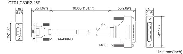
Model nameL (mm (inch))RemarksGT01-C30R2-25P3,000 (118.11")RS-232 cable for direct connection to FXCPU special adaptor<br/>(25-pin D-sub)
