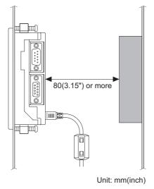
Cable protrusion dimension
