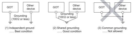
• Set the grounding point closer to the GOT to make the grounding cable short as possible. Provide grounding using a single grounding wire. Refer to the table below to select the proper size grounding wire.
