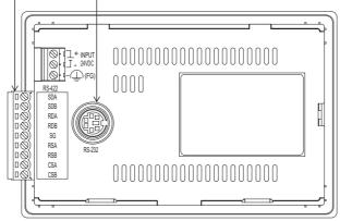
Whether an RS-422 or an RS-232 interface (Standard I/F-1) for communication with PLC is used depends on the GOT model.
