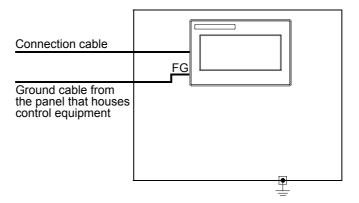
If electric potential difference between the ground points created by it causes malfunctions, lowering the voltage as shown in Remedy 1 below may solve the problem.
