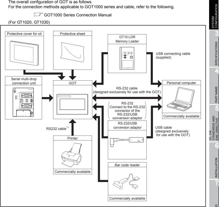
The RS-232 cable vary depending on the specifications of the user's printer. Use the RS-232 cable according to \*1: the specifications of the user's printer. Only hard copy of the screen can be printed.
