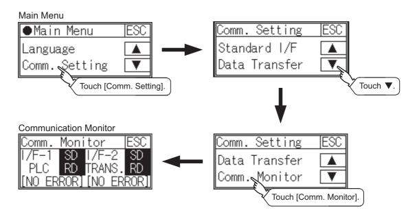
Communication Monitor (When bar code is connected)
