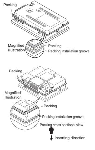
Inserting into the panel face
