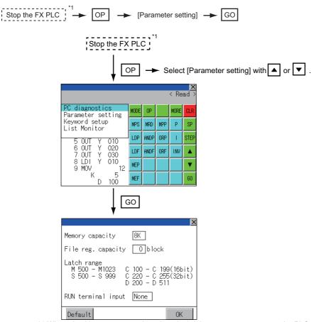
\*1 When checking parameters (not changing), it is not necessary to stop the PLC.
