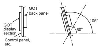
• The GOT will have a longer lifetime if used within the mounting angles shown above. Ideally, the temperature inside the control panel should not exceed 0 to 40°C
