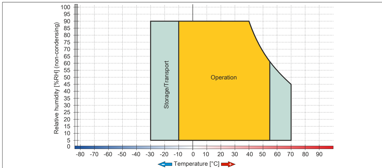
Figure 62: 5AP933.240C-00 ≥D0 - Temperature/Humidity diagrams
