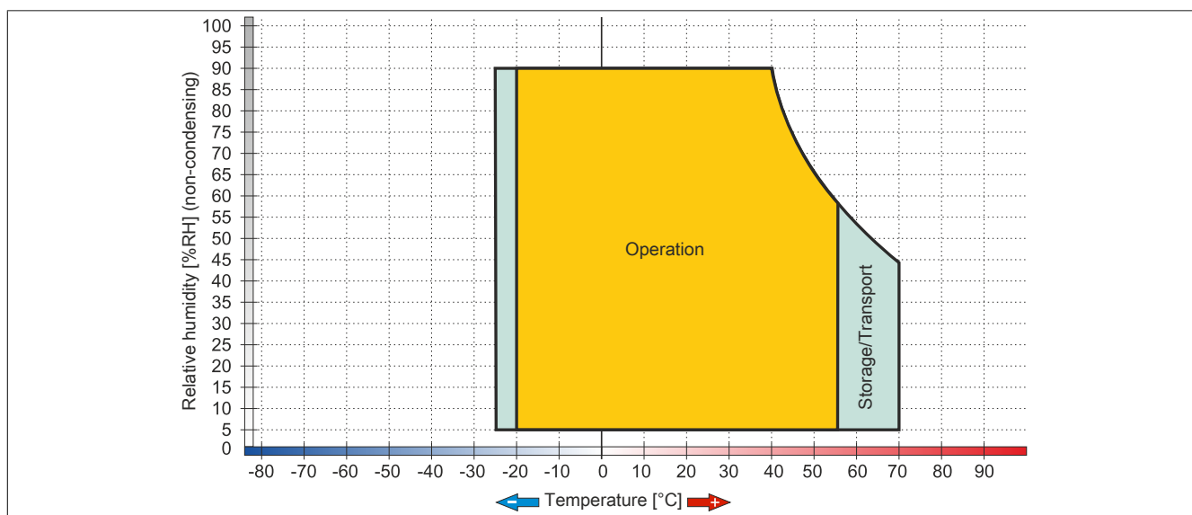
Figure 97: 5AP1120.156B-000 - Temperature/Humidity diagram
