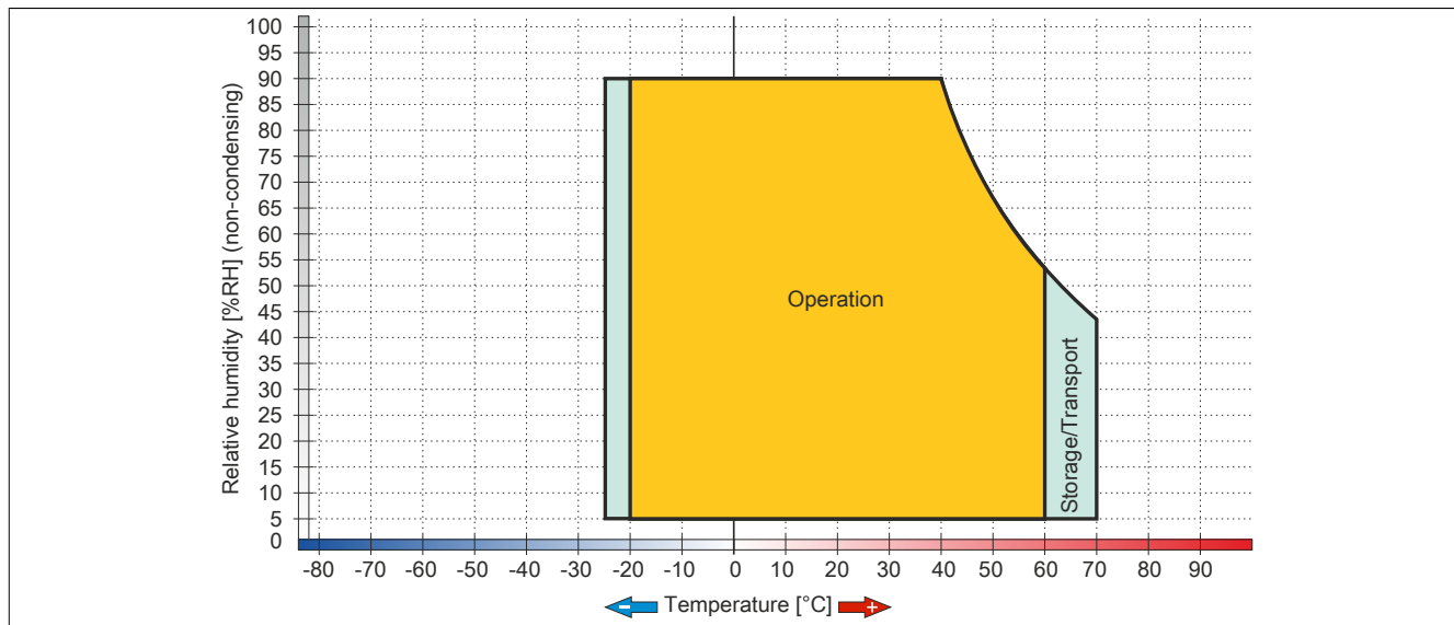
Figure 50: 5AP923.1906-00 ≥Rev. E0 - Temperature/Humidity diagram
