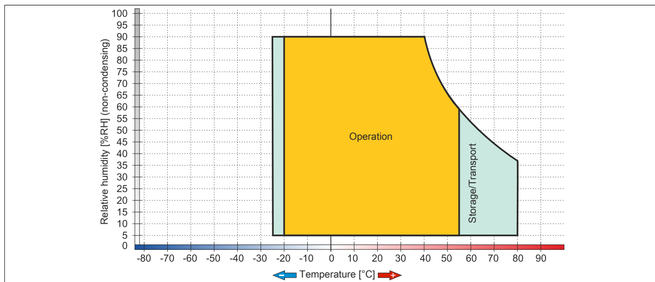
Figure 76: 5AP1120.1043-000 - Temperature/Humidity diagram
