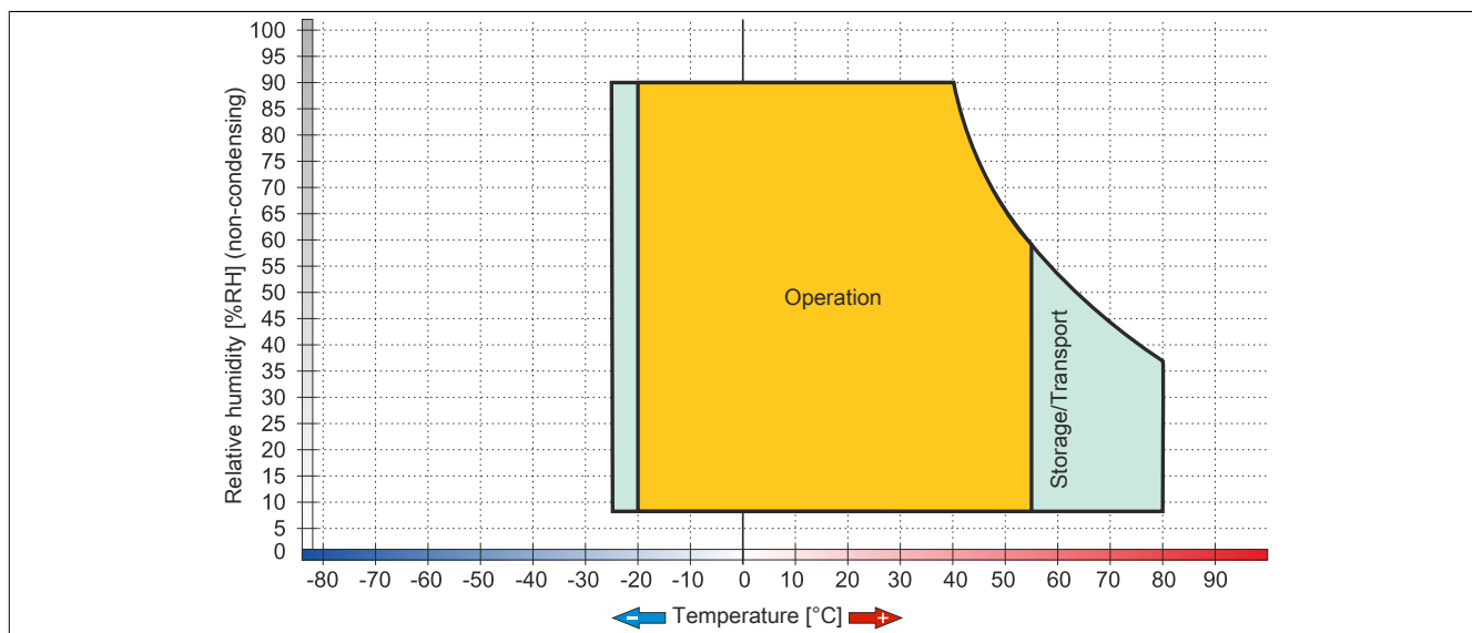
Figure 92: 5AP1180.1505-000 - Temperature/Humidity diagram
