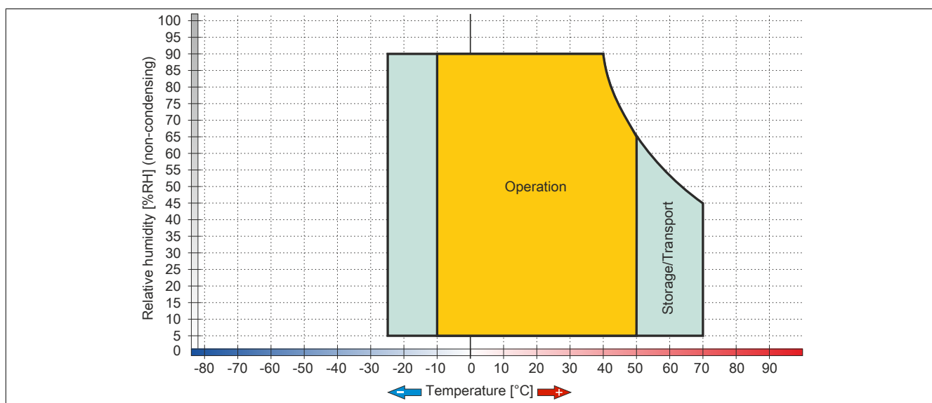
Figure 101: 5AP1130.185C-000 - Temperature/Humidity diagram
