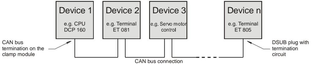
If the terminal is an end module, it can be terminated by placing a 150-Ohm resistor between CAN-A (Low) and CAN-B (High).
