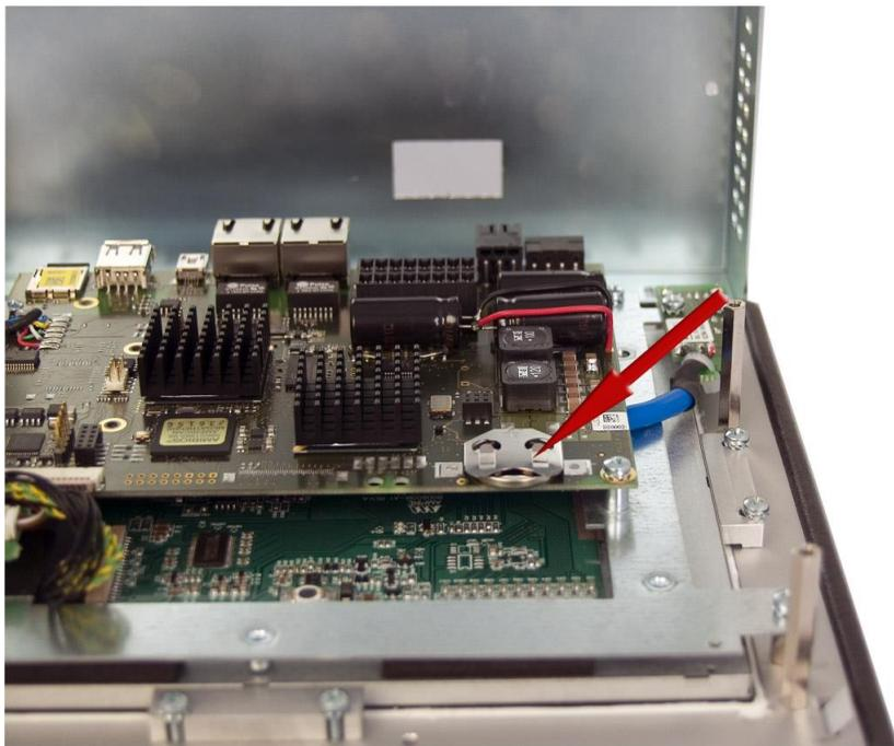
4. Using the strap, remove the battery the holder (see arrow).
