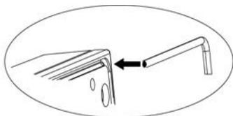
① Sponge rubber band should be inserted in the groove provided on the back of the terminal.
