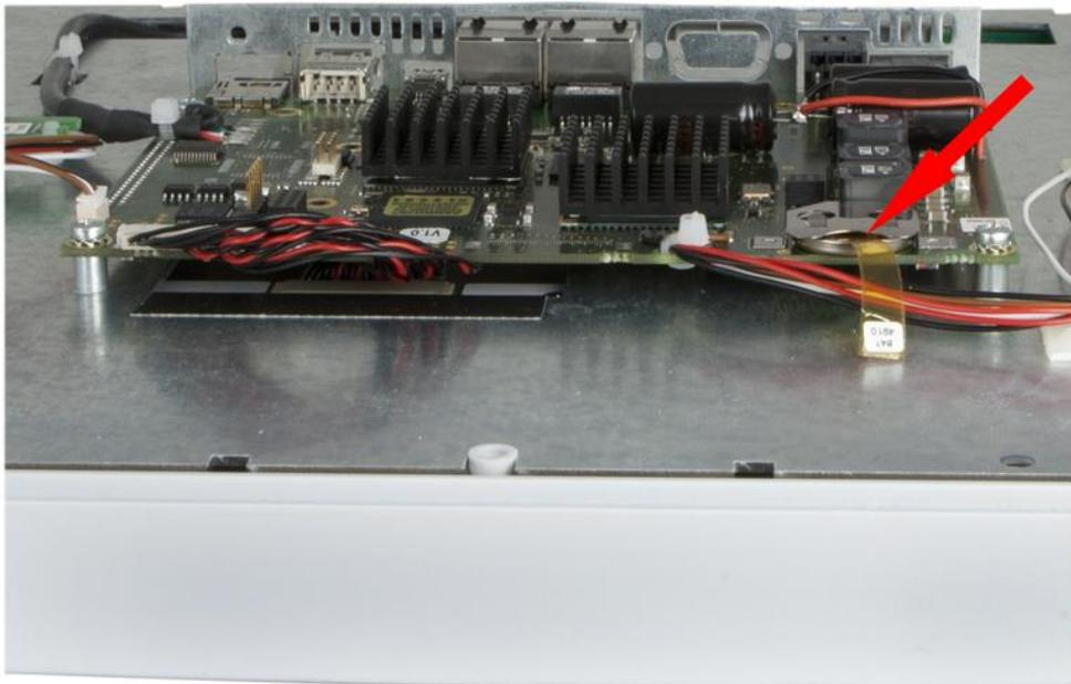
4. Using the strap, remove the battery the holder (see arrow).
