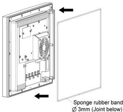
② Incorporate section with the switch cabinet. Connect the terminal with the supplied screws.
