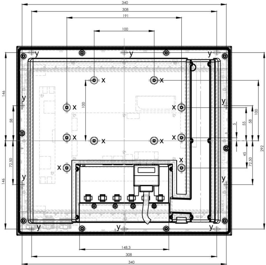
x => mounting holes for carrier arm mount(10x).
