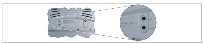
The Power Panel 65 is equipped with 2 hex switches that can be used as operating mode or node number switches. Switch positions 0x01 to 0xFE are used to set the INA node number of the Ethernet interface.
