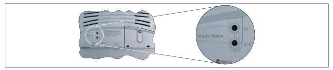
The Power Panel 65 is equipped with 2 hex switches that can be used as operating mode or node number switches. Switch positions 0x01 to 0xFE are used to set the INA node number of the Ethernet interface.
