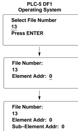
3. Enter the PID file number and word or element / sub-element address.
