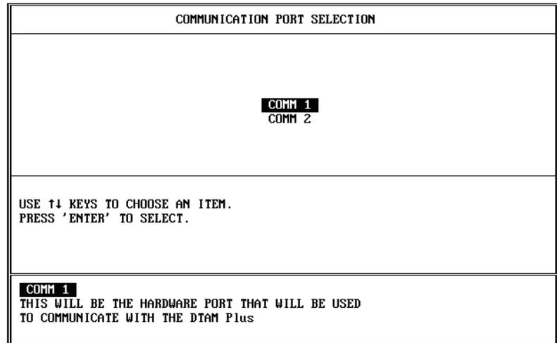
9. Highlight the serial port on your computer that is connected to the DTAM Plus (COMM 1 or COMM 2) and press [Return].
