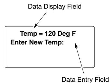
The data entry field must always appear last on the screen. The application designer cannot place text after a data entry field.
