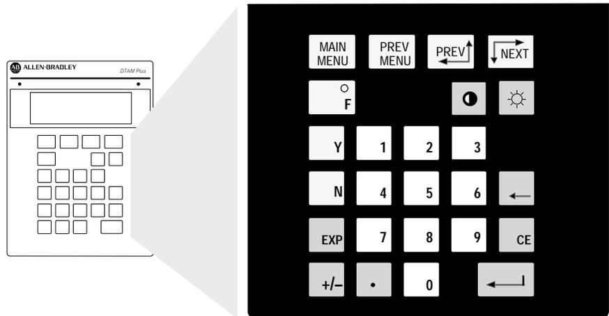
The keys on the DTAM Plus keypad are color coded by function. Blue keys are for navigation and operator responses; dark grey keys control display and format; and light grey keys are for numeric entry.
