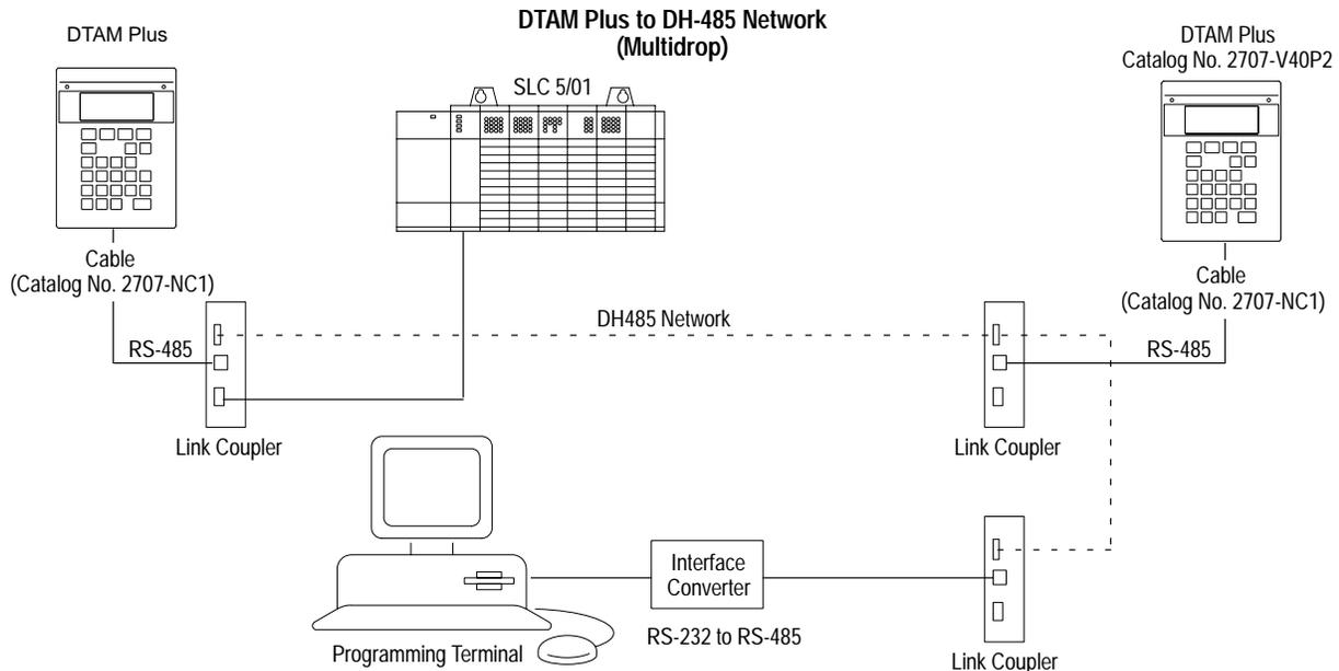
**To connect the DTAM Plus terminal to an RS-485 device:**
