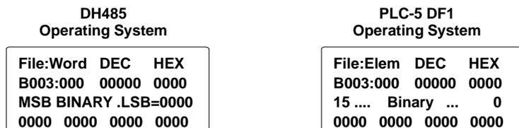
4. To change a value or the element address, move the cursor into the data field using the [NEXT] or [PREV] keys. Enter the new data. If you are editing binary data, use the [+/-] key to toggle the data between 1 and 0 and press [NEXT] or [PREV] to move to the next bit.
