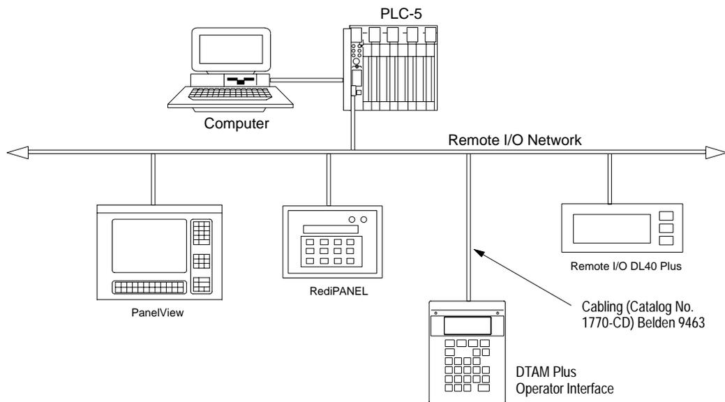
**DTAM Plus to an SLC 5/03, 5/04, 5/05 Remote I/O Scanner**
