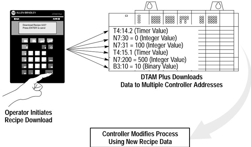
Depending on how the application was designed, recipe screens will either automatically download data or display a prompt allowing the download to be initiated when [Y] is pressed.
