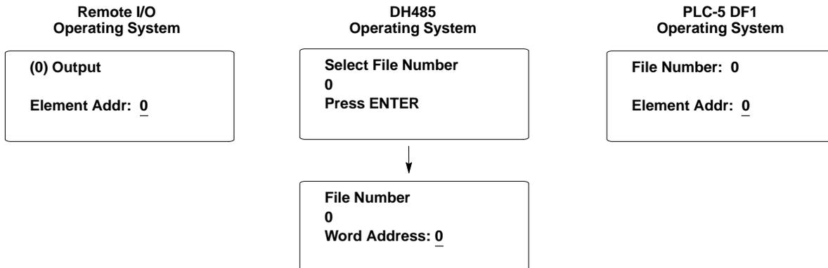
3. Enter the Element Address (PLC) or the File Number and Word Address (SLC) If you are accessing PLC data, you must enter an octal value.
