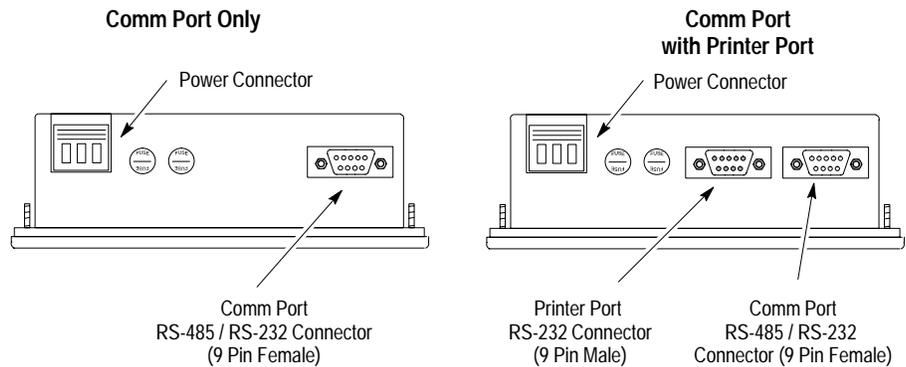
The DTAM Plus supports the following parameters for RS-485 and RS-232C communications:
