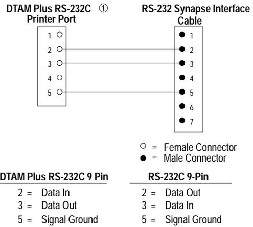
① The communications port of the DTAM Plus must be set to RS-232.
