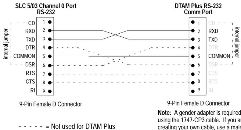
The control lines (pins #1, #4, #6, #7, and #8) are not used by the DTAM Plus. The connections to these pins can be deleted for this application.
