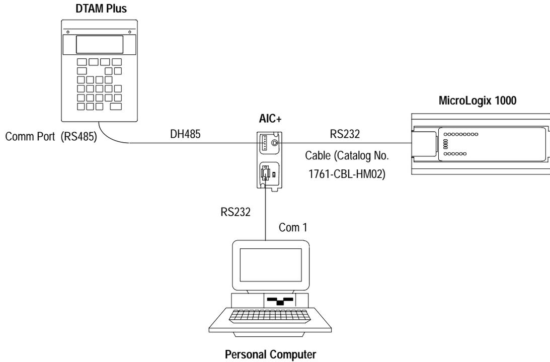
You will need to construct a cable that connects to the AIC+ and the DTAM Plus/Micro. Refer to the following illustration.
