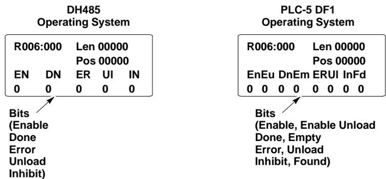
4. To change the Len and Pos values or element address, move the cursor to the data field using the [PREV] or [NEXT] keys. Enter the new data.
