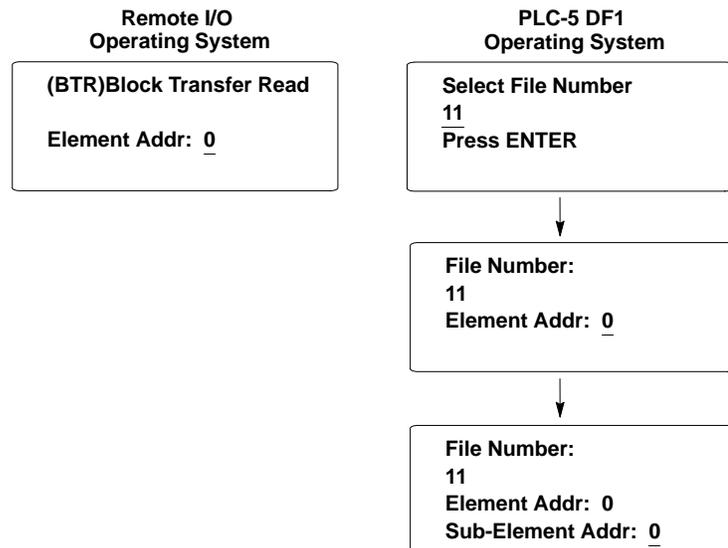
3. Enter the block transfer file number and word or element / sub-element address.
