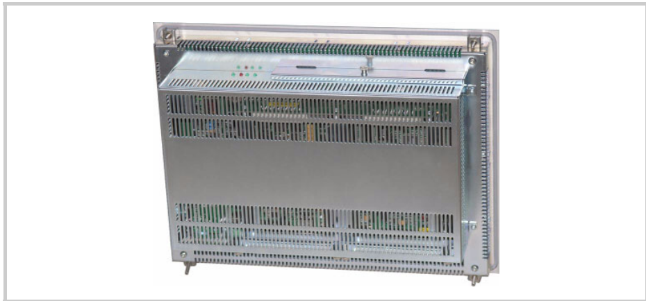
Fig. 41 10.4" and 12.1" devices with four retaining brackets (do not meet IP65 requirements)
