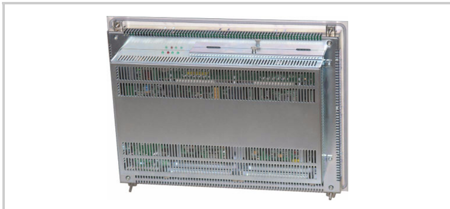
Fig. 27 10.4" and 12.1" devices with four retaining brackets (do not meet IP65 requirements)
