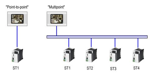
Modbus protocols use station addresses (STx). Accordingly, both "point-to-point" and "multipoint" connections can be implemented when using the appropriate physical interface (see the figure above).
