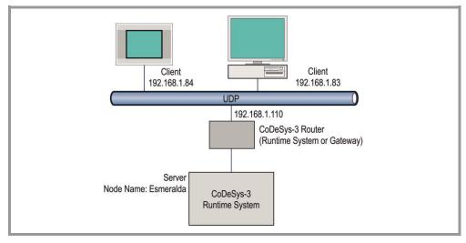
Fig. 22 How it works with a CODESYS V3 router
