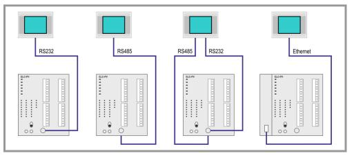
Fig. 51 How it works with panels
