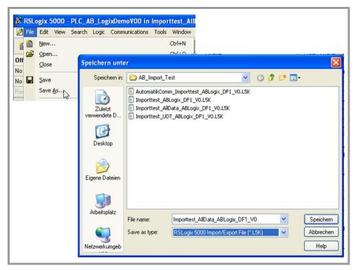
Fig. 38 Example of tag export from RSLogix 5000 in the L5K format
