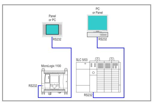
Fig. 30 How serial communication works
