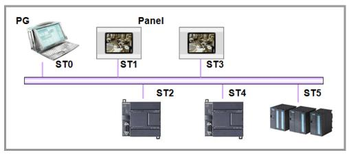
Fig. 79 How the panel works on an MPI/PROFIBUS-DP network
