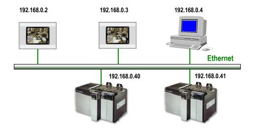
The station and IP addresses shown above are examples. What is important is for each individual node to be assigned its own unique station and/or IP address.
