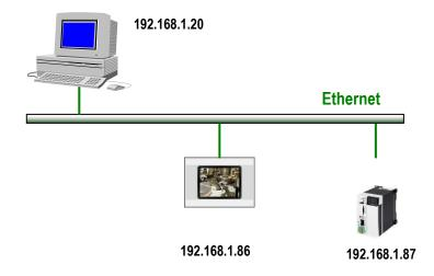
Note: The IP addresses used here are only an example! What is important is for each individual device to be assigned its own unique IP address.
