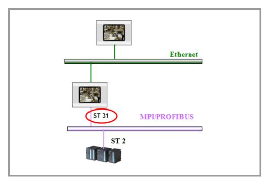
Fig. 71 Station numbers - Station 2 and panel 31
