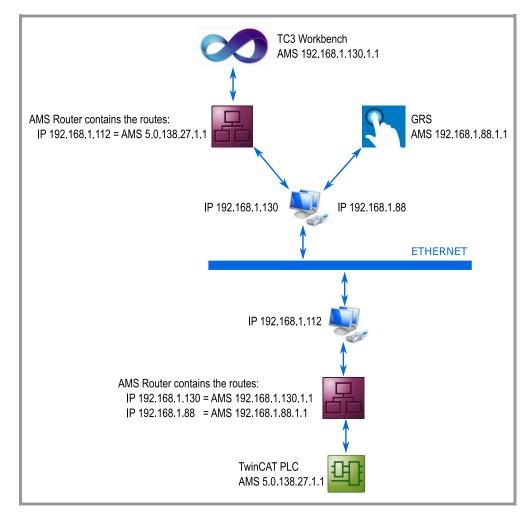
Fig. 94 Example showing a schematic view of how to setup up the IP addresses in order to run GRS and the TC3 Workbench on the same PC.
