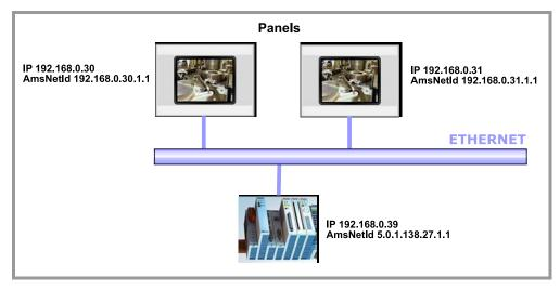
Fig. 84 Example shows how IP addresses and AmsNetId's are addressed within a setup connecting two panels with a Beckhoff TwinCAT device over Ethernet.
