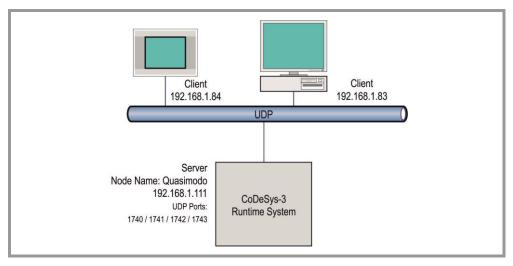
Fig. 21 How it works without a CODESYS V3 router
