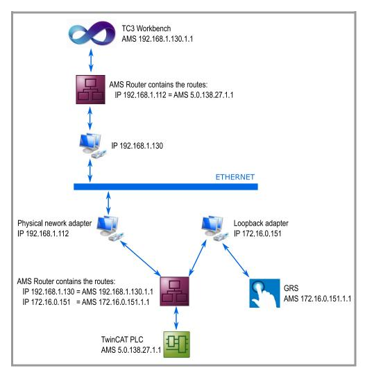
Fig. 92 Example showing a schematic view using a physical network adapter together with a loopback adapter on the same PC in order to allow GRS to have its own AMSNetId.
