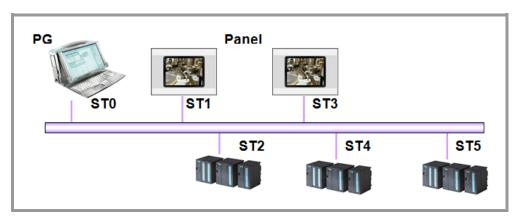
Fig. 58 How the panel works on an MPI/PROFIBUS-DP network
