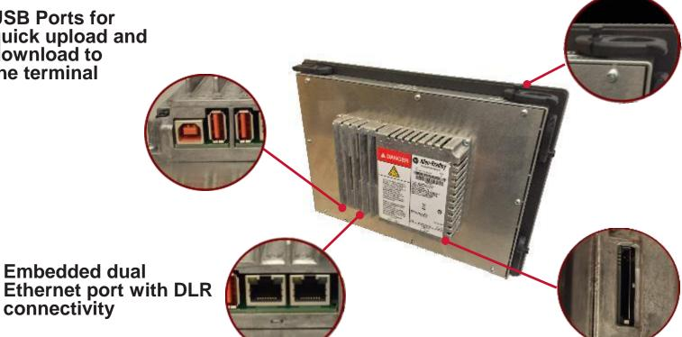
**New installation clamps** provide fast and simple terminal installation and removal
