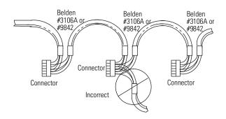
Attach the connector to the Belden #3106A or #9842 Cable as shown below.
