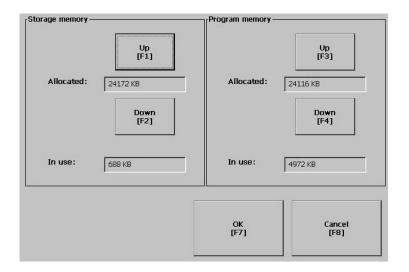
You can modify the allocation of storage or program memory. Press the **Up** or **Down** button to increase/decrease the memory allocation. Each button press changes the allocation by a value of 4. If you change the allocation for one type of memory, the other is automatically updated accordingly.
