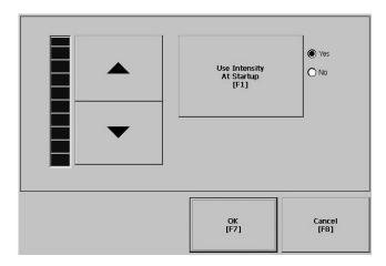
The screen indicates whether the current intensity of the backlight will be used when the PanelView Plus terminal starts up. The button toggles between Yes or No.
