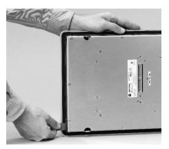
The legend inserts for the K1-Kxx function keys on the left and right side of the display are accessible when the Display Module bezel is removed.
