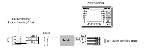
The orientation of the Remote I/O Connector on the PanelView Plus is reversed from the PLC Scanner connector. However, the polarity is the same as the scanner card connection to the SLC.
