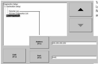
To access the Remote Log Setup or Message Routing, select the node and then the Edit button.
