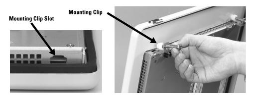
**6.** Tighten the clip mounting screws by hand until the gasket seal contacts the mounting surface uniformly.
