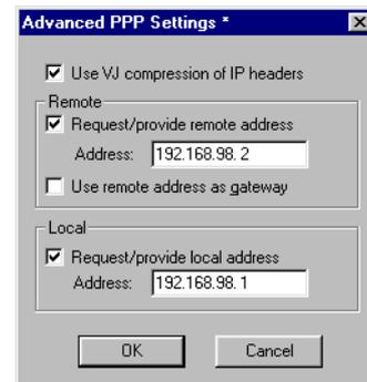
Settings under TCP/IP, IP Address, Subnet mask and Gateway, are of no importance in this case. PPP will change parameters.
