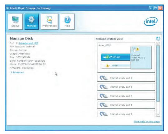
Figure 7-4 Information about the functioning hard drive
