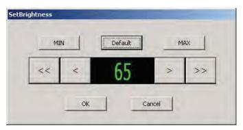
Set the brightness ""Brightness" of the screen via the backlighting. The factory setting and the "default" value is 65. Call via an icon on the desktop.
