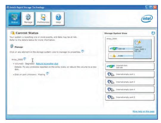
Figure 7-5 Restoring the RAID system
