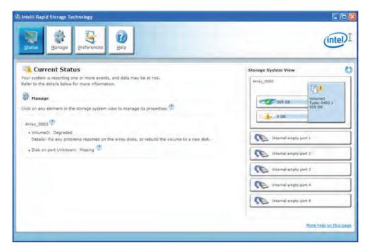
Figure 7-3 Degraded message of RAID software
