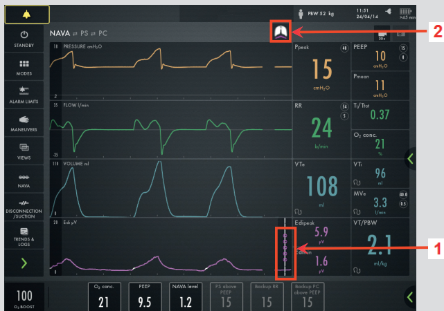
NAVA mode screenshot from actual patient ventilation. The shortcut to Edi catheter positioning 1 .
