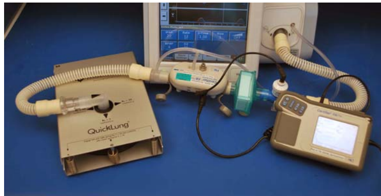
Figure 8-20: Oxygen Accuracy Test Configuration
