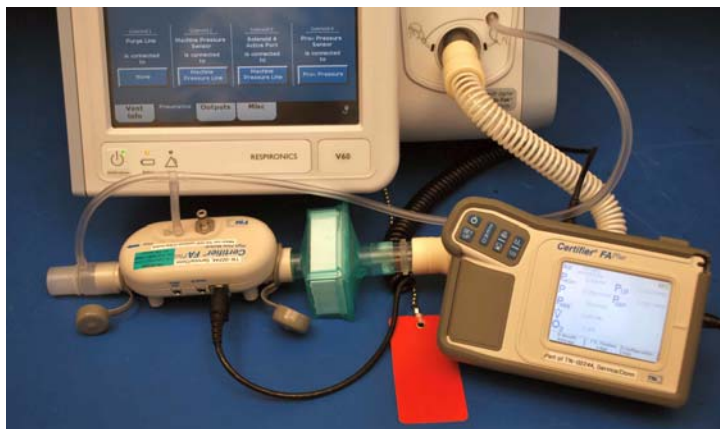
Figure 8-18: Air Flow Accuracy Test Configuration
