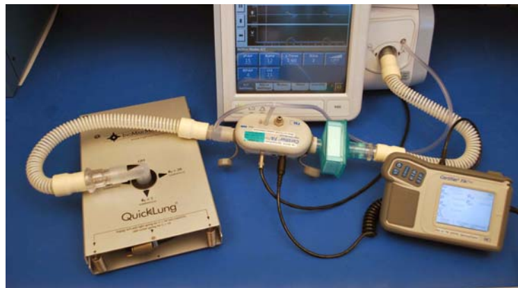
Figure 8-21: S/T Performance Test Configuration
