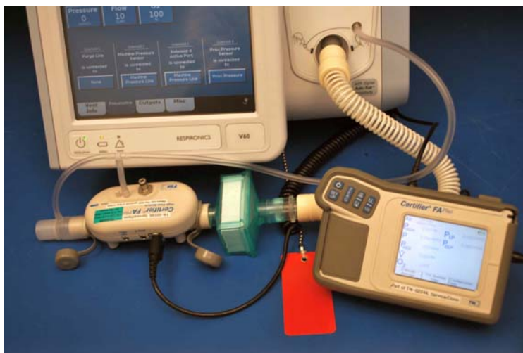
Figure 8-19: Oxygen Flow Accuracy Test Configuration
