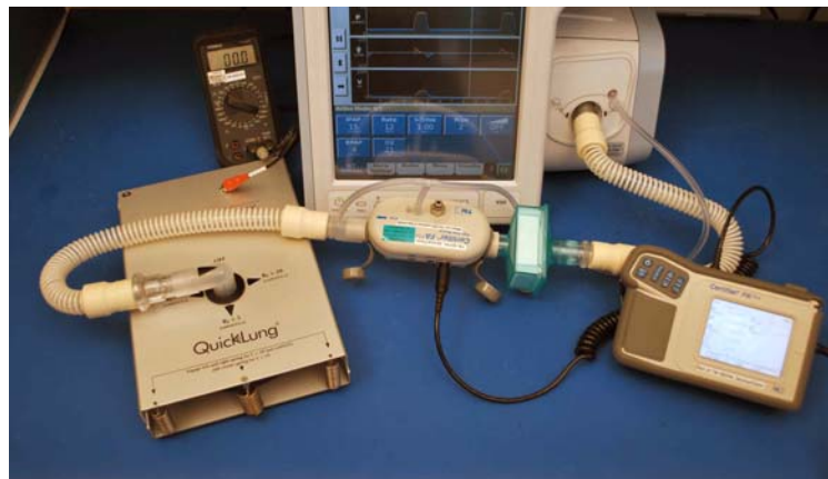
Figure 8-22: Alarms Test Configuration
