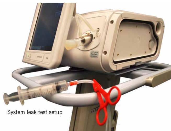
Figure 8-11: Leak Tests Configuration
