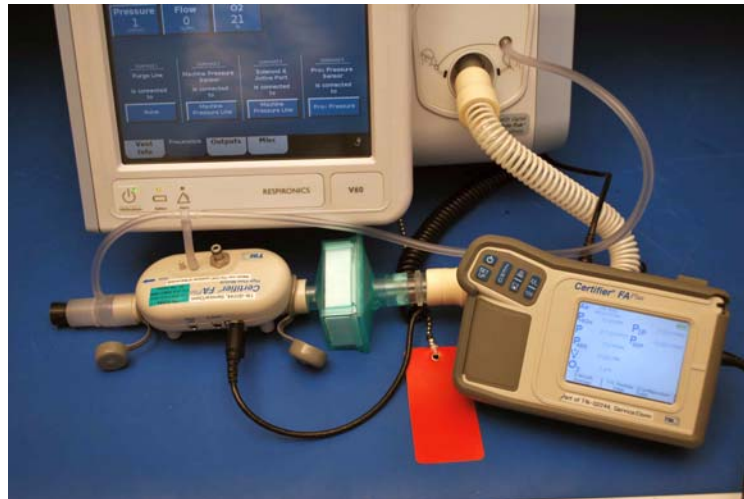
Figure 8-15: Pressure Accuracy Test Configuration
