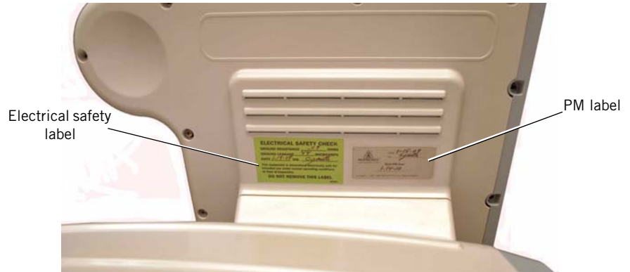
Figure 4-6: Electrical Safety and PM Label Placement
