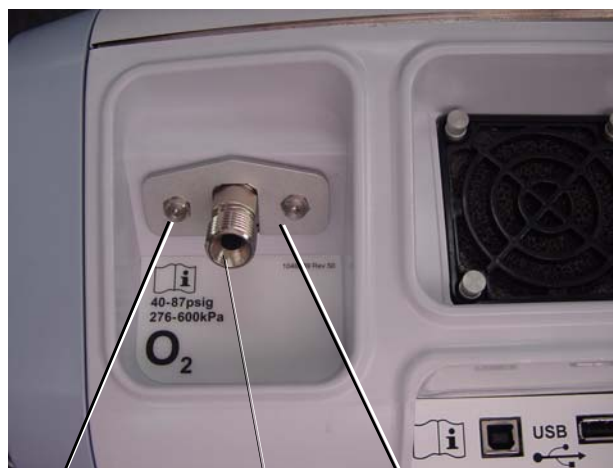
M3 screw (x2) (113 ± 11.3 N cm/ 10 ± 1 in.-lbf) Washer (x2) Oxygen inlet Retaining bracket
