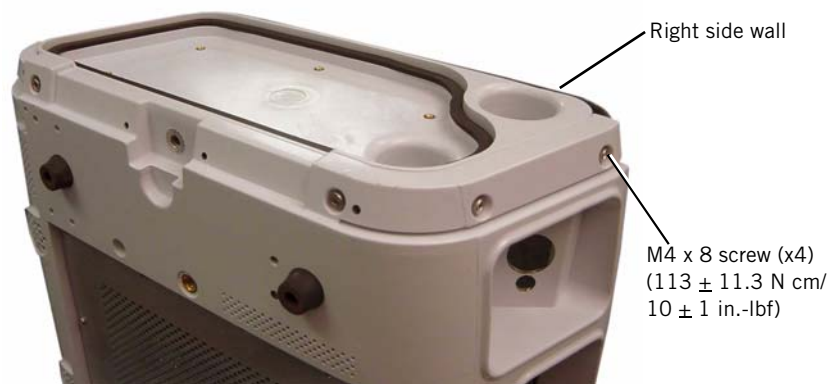
Figure 7-22: Removing the Right Side Wall
