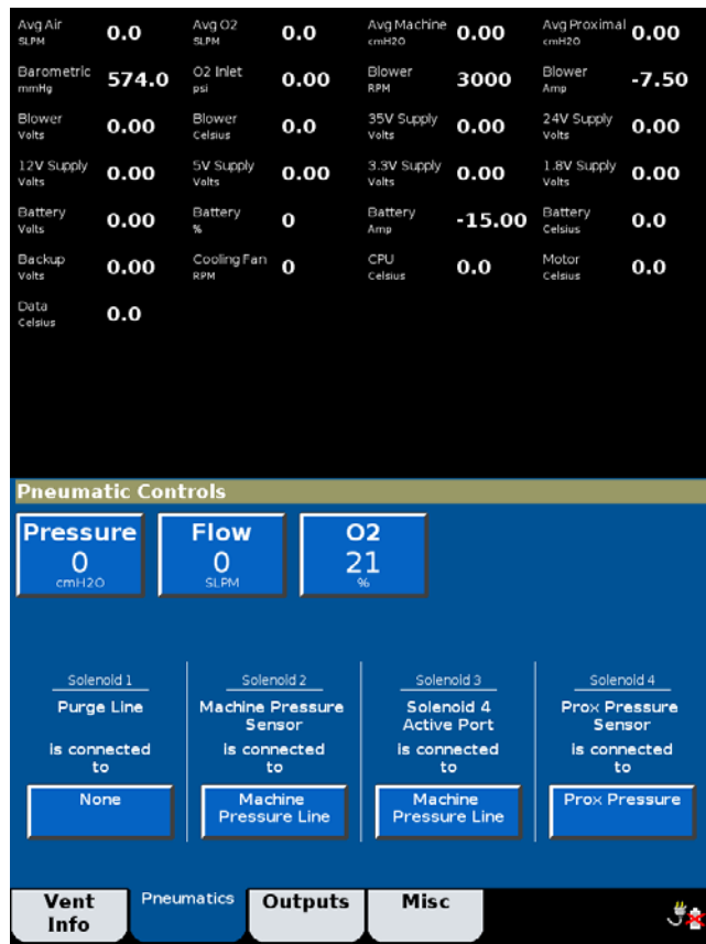
Figure 5-11: Pneumatic Controls Screen
