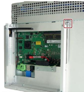
4. Insert the PCIe card in the direction of the arrow and secure this with the marked screw.
