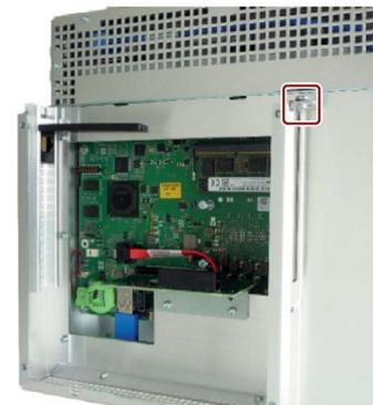
5. Push the PCIe card holder in the direction of the PCIe card and secure this with the marked screw.
