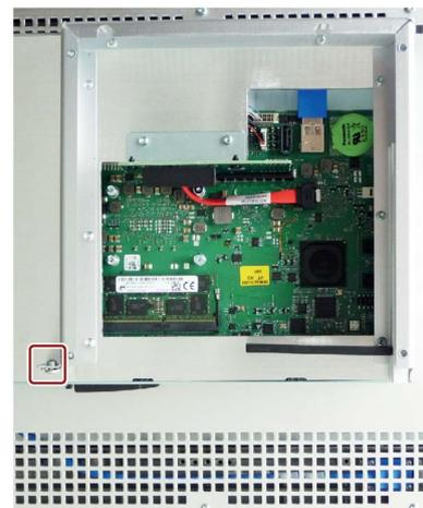
3. Loosen the marked screw of the PCIe card holder and remove the masking frame.
