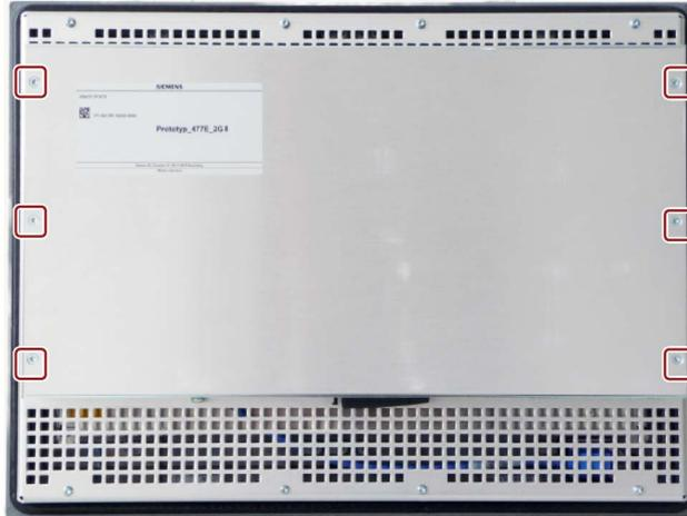
Position and number of the fastening screws are the same for the devices with 15", 19" and 22" display.
