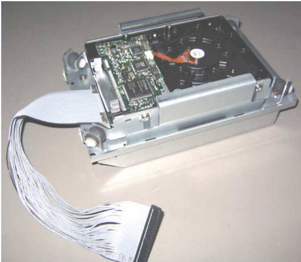
Figure 12-8 Removed hard disk
