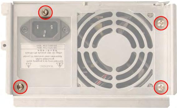
The image shows the rear view of a power supply unit (PSU) mounted in a chassis. On the left side, there is a power input socket with two screws. To the right of the socket is a large circular fan. Four screws are circled in red, indicating they are the ones to be removed: one at the top center, one at the top right, one at the bottom left, and one at the bottom right. A warning label is visible below the power socket. |
