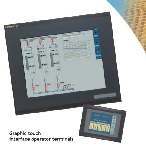
This group includes displays of 3.8", 5.7" and 10.4". The smallest is a black and white terminal with built-in Ethernet and backlight dimming. The 5.7" display terminals range from gray-scale STN-LCD to 256-color TFT-LCD, and the 10.4" TFT-LCD display terminals includes one with 100-240 V AC, and one with +24 V DC power supply. The 3.8" and 5.7" terminals can be mounted either horizontally or vertically.
