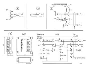
Some (older) operator panels had pull-up and pull-down resistance except for the actual bus termination at  $120 \Omega$ , similar to Westermo and Profibus. See 1 in drawing above.
