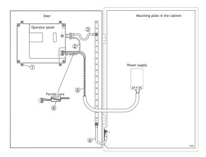
The operator panel's mounting clamps do not provide a secure grounding connection between the panel and the device cabinet, see 1 in drawing above.
