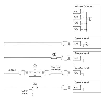
In some industrial units for Ethernet, the RJ45 contact's shield is connected to the chassis via a capacitor, see 1 in drawing above.
